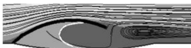
Fig.2. Calculated aggregation zone in the venous valve model at the minimum flow instance
